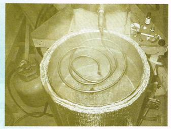
A perforated copper coil serves as a sparge water sprinkler.
