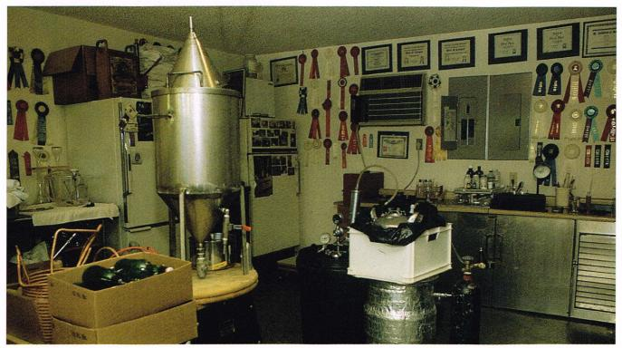
George's homebrewery is more laboratory than kitchen. There is a one-half-barrel Unitank cylindroconical fermenter, counterpressure bottle-filling equipment in the foreground and wild yeast and bacterial detection media, microscopes and a hemocytometer on the counter.
