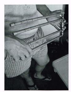
Ray explains that the slotted copper pipe fits into a picnic cooler he has converted to a mash tun. The slotted pipe allows sweet wort to drain into the kettle while leaving the spent grain behind.
